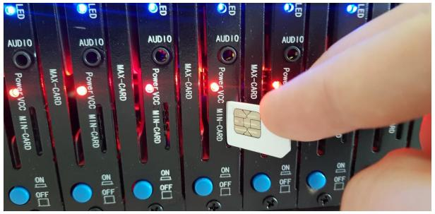
After inserting a SIM card please remember to turn modem's switch to ON.
